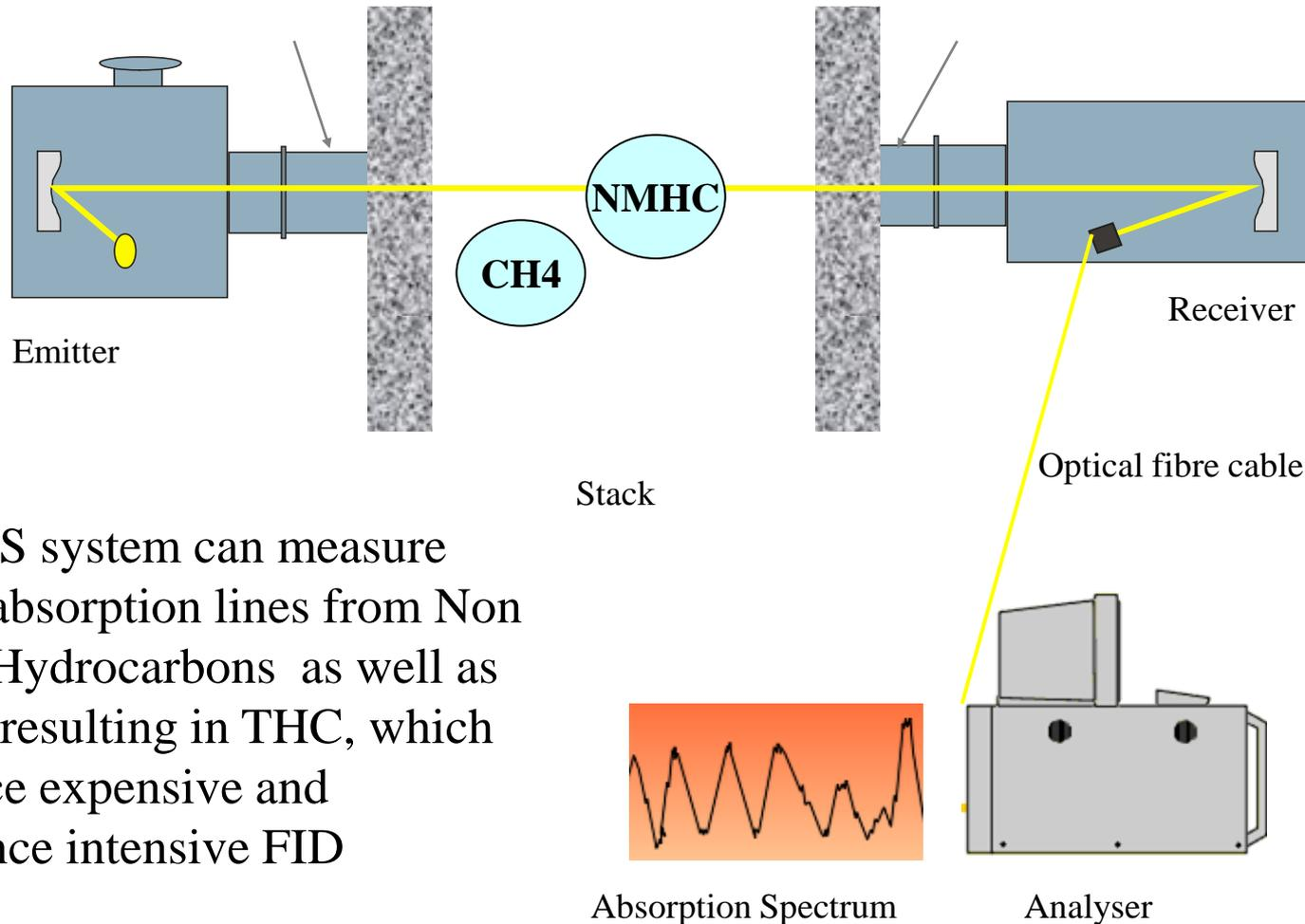
The DOAS system can measure common absorption lines from Non Methane Hydrocarbons as well as Methane, resulting in THC, which can replace expensive and maintenance intensive FID analysers.
